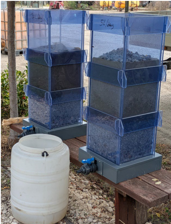
Figure 16: Filled filter columns with 50-liter greywater tank. The left column is filled with coarse sand and can be loaded with 20 liter per day, the right column with fine sand and can be loaded with 5 liter per day.
