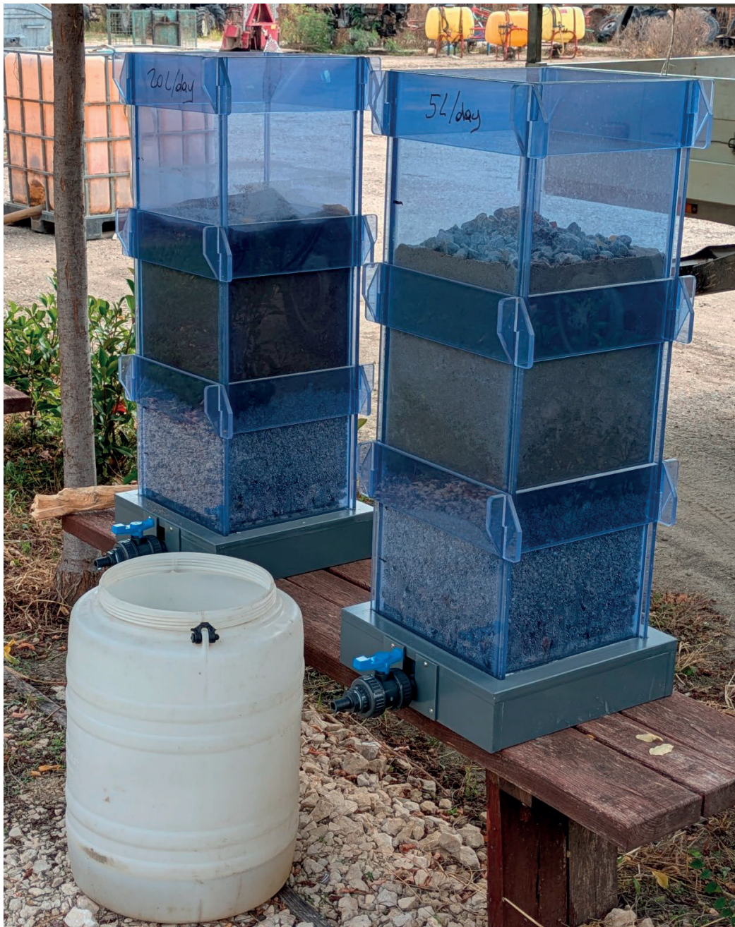
VF wetland models with 50-liter greywater tank.
