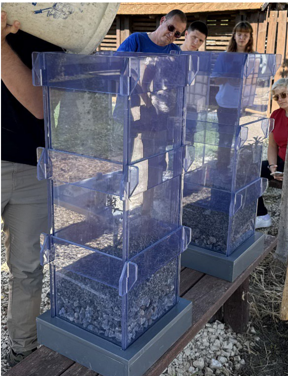
Figure 6: Filling of intermediate layer
