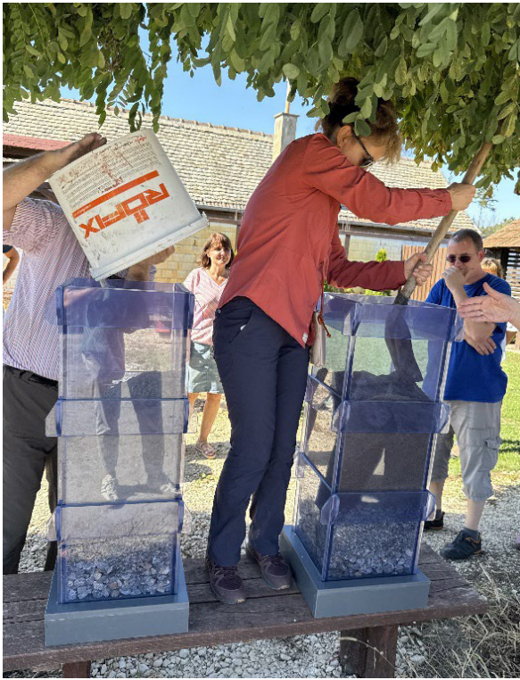
Figure 8: Filling of main layer (left column) and making a flat filter surface (right column)
