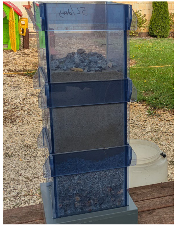
Figure 9: Filled filter column with coarse gravel on top
