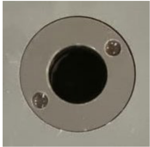
Figure 6: Adapted standard part-holes for angle grinder key
