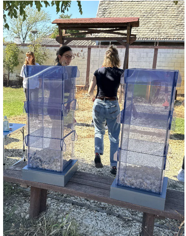
Figure 5: Filter columns with drainage layer
