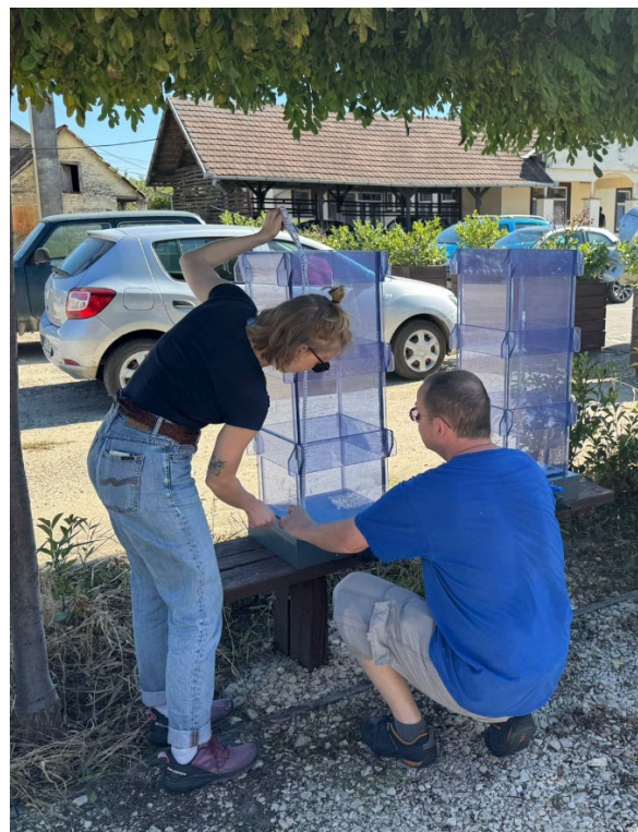
Figure 3: Marking the height of the filter layers with a marker
