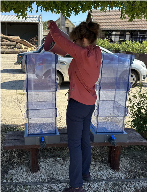
Figure 4: Filling of drainage layer
